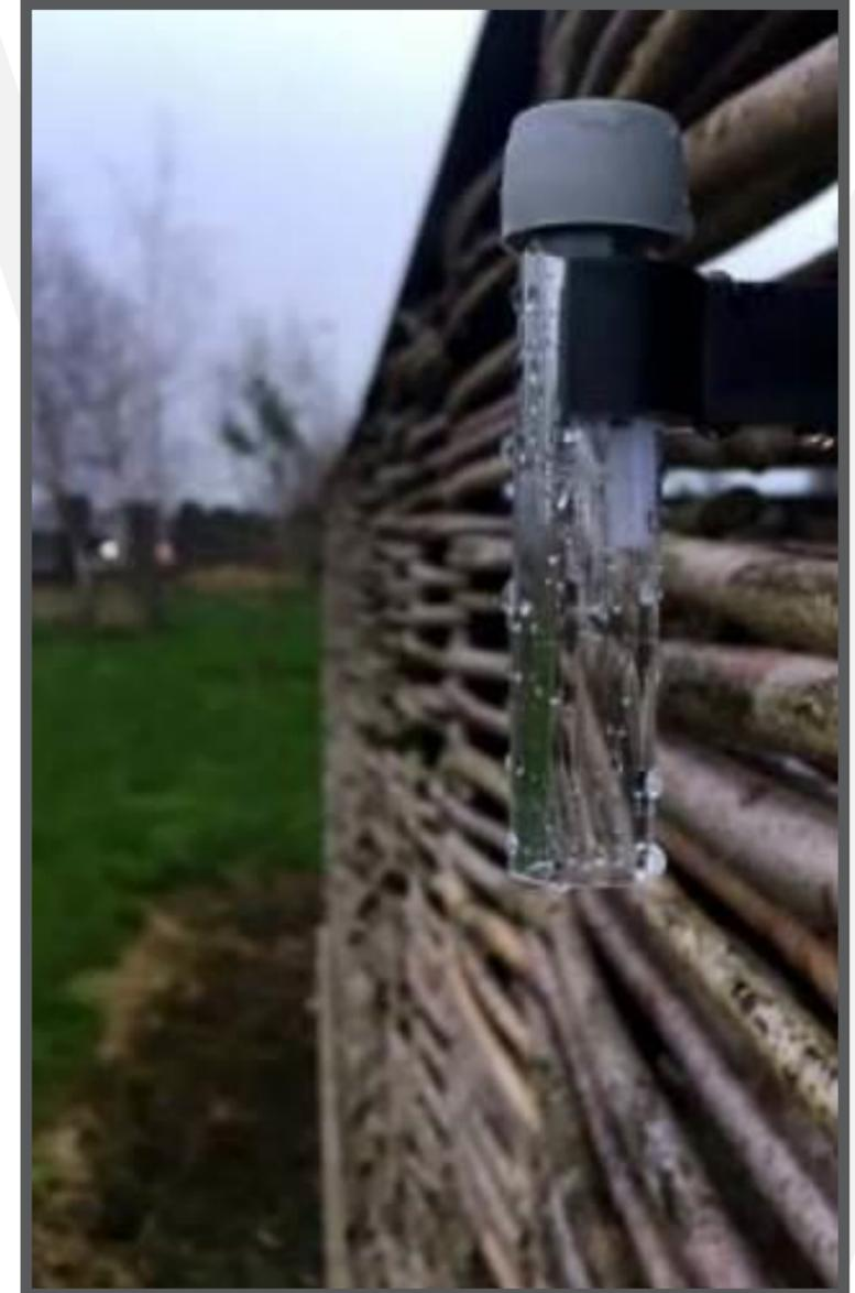
Nitrogen Dioxide diffusion tube monitoring along M50
