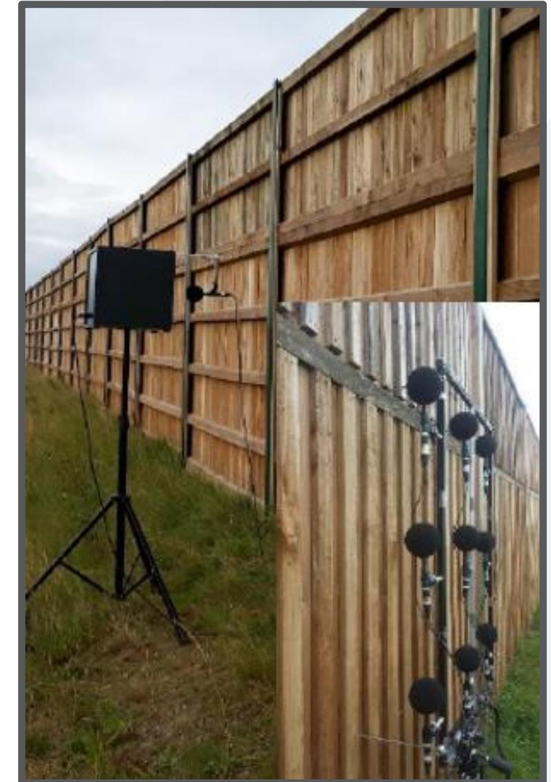
*In situ* acoustic testing of a reflective environmental noise barrier on M17/M18
