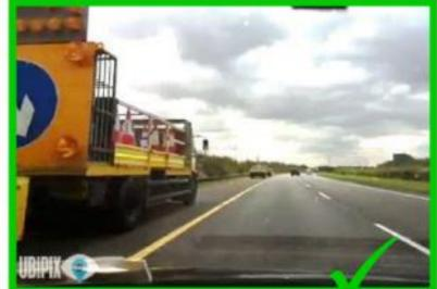
Where there is a risk of traffic entering the area between the block vehicle and the working vehicle, the distance between these vehicles should be 50 metres.
