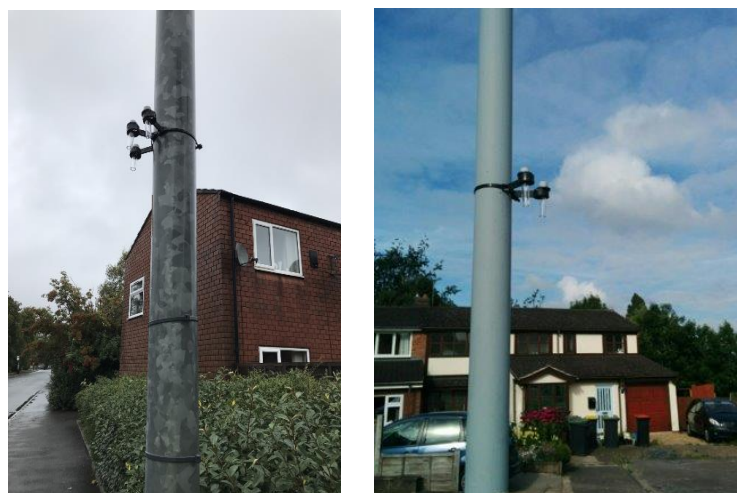
Figure 3.12 Examples of Diffusion Tube Set Up
