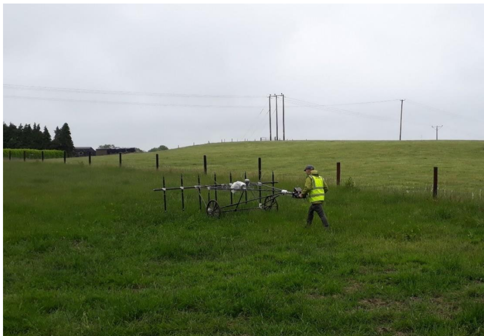
Plate 5.6 - Geophysical surveying to detect subsurface archaeological features (Photo: TII)
