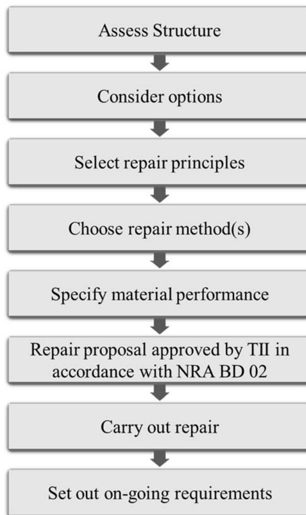
Figure 2: Key Steps in the Repair Process
