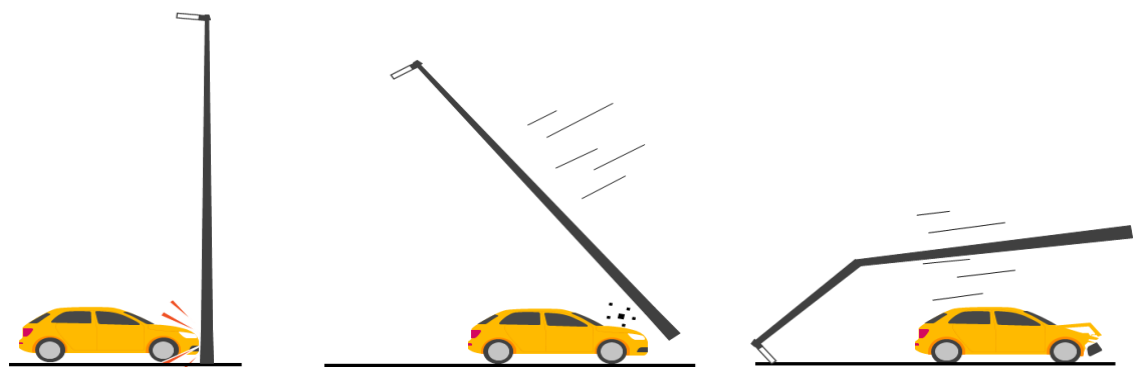
Figure 4.4 Behaviour of a non-energy absorbing (NE) column
