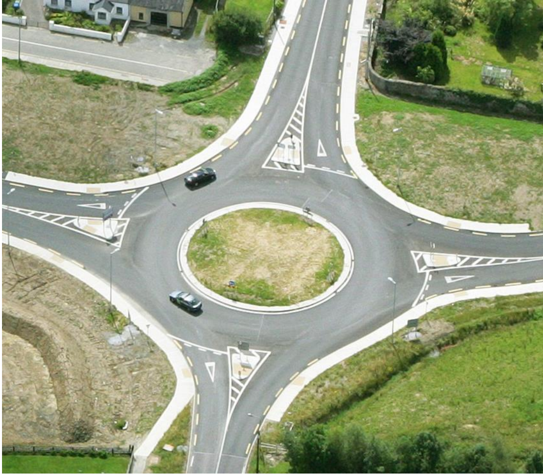
Figure 2.6 Single Lane Roundabout
