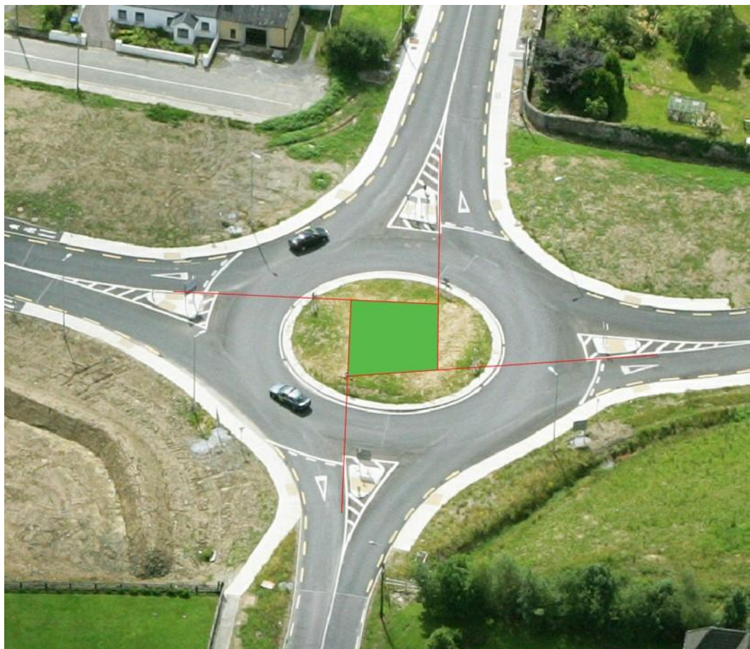
Figure 6.4 Permitted location for non-passively safe landscaping and artwork within a single lane roundabout
