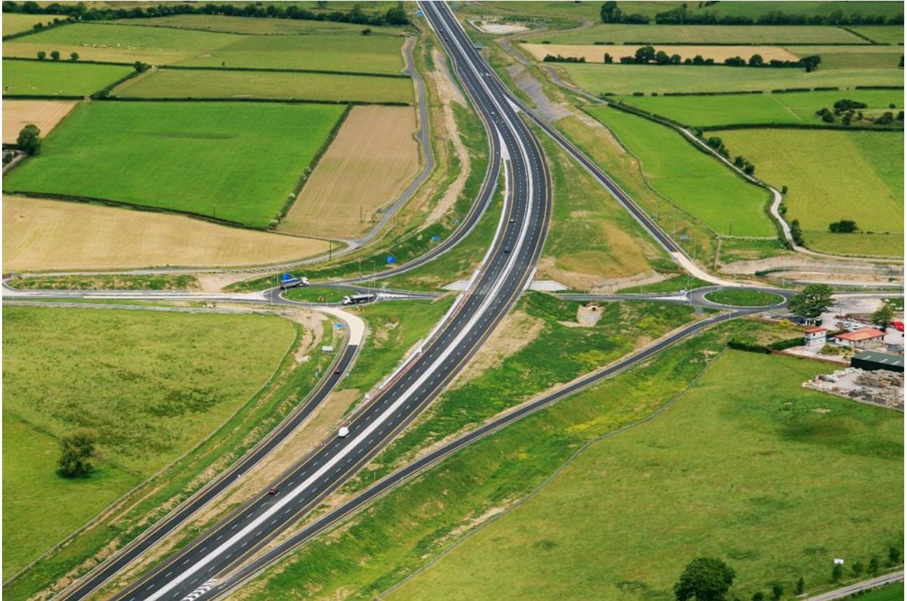
Figure 2.8 “Dumb-bell” Grade Separated Junction
