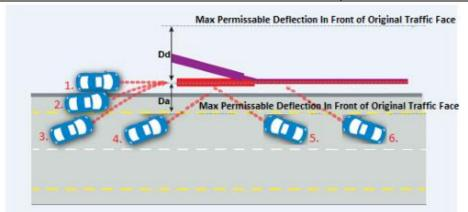
\*Refer to Figure 4 of CEN/TS 1317-7:2023 for details of Vehicle Approach Paths and Impact Angles \*\*Refer to Table 1 of CEN/TS 1317-7:2023 for details of required tests for the performance class
