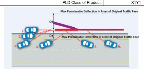
\*Refer to Figure 2 of prEN 1317-7:2014 for details of Vehicle Approach Paths and Impact Angles
