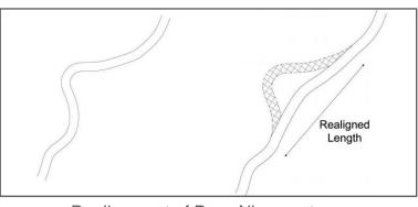
Realignment of Poor Alignment
