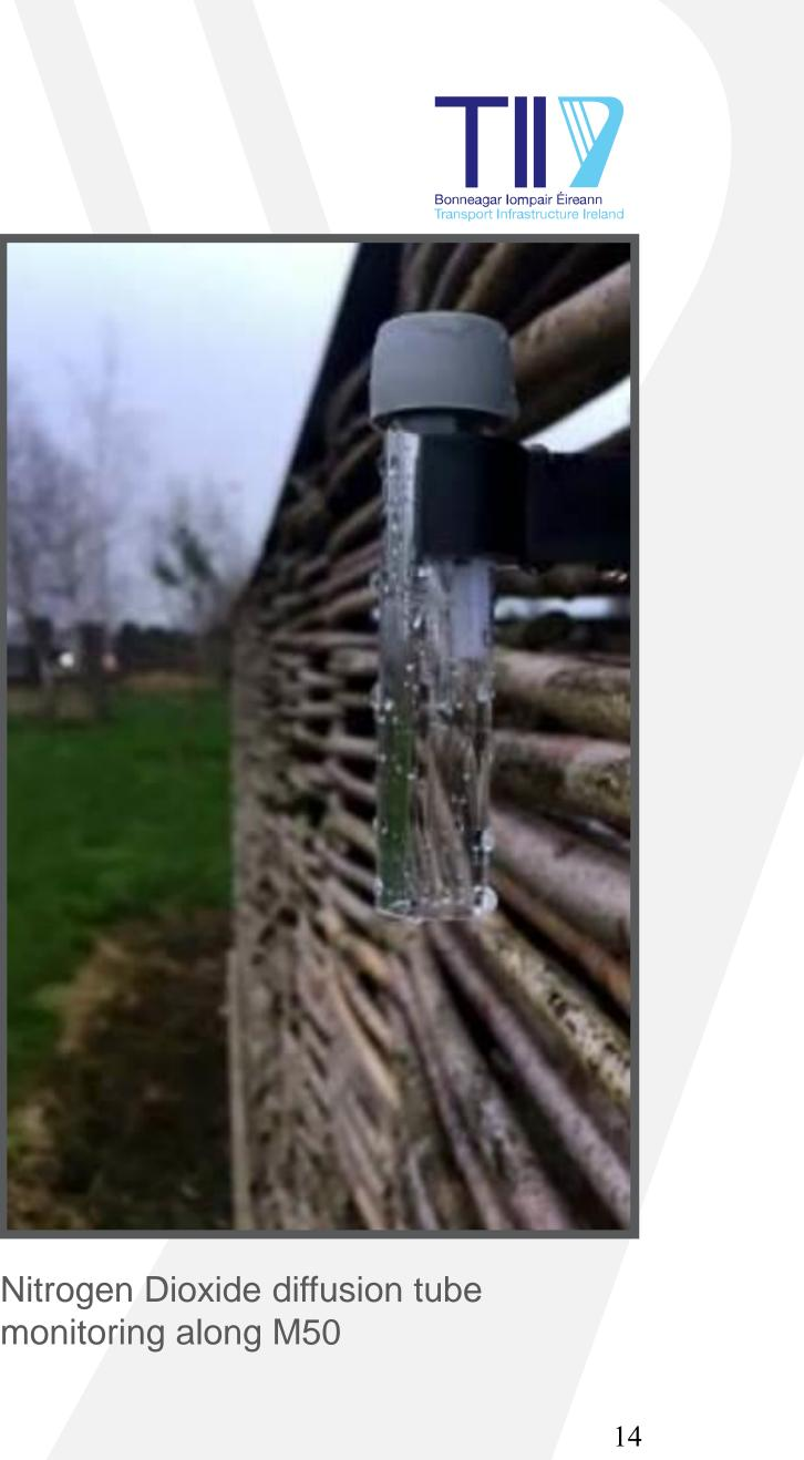
Nitrogen Dioxide diffusion tube monitoring along M50
