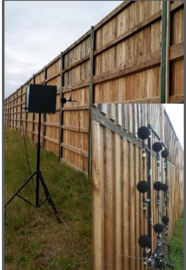
In situ acoustic testing of a reflective environmental noise barrier M17/M18
