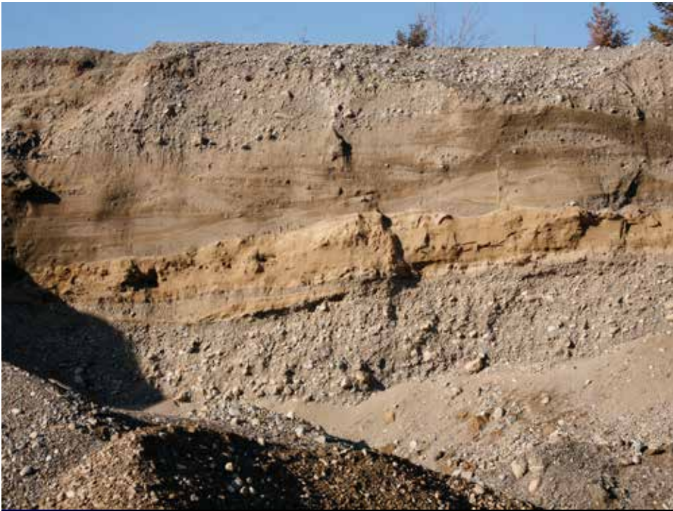
Plate 12 Glacial Sub soils with a variety of permeabilities. The nature and thickness of the subsoil determines the vulnerable rating of the underlying aquifer. Glacial subsoils can have a large variety of permeabilities indicating the importance of local site investigation.
